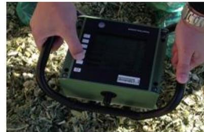
Figure 2. Ejkelkamp Penetrometer
